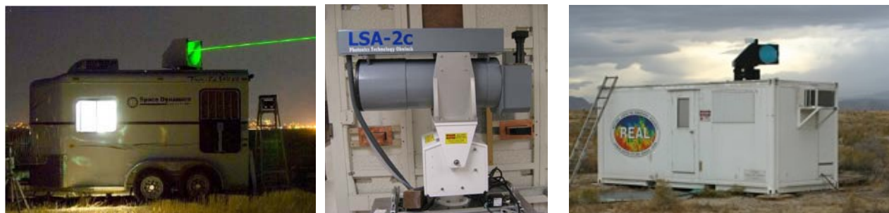
Figure 5. left to right, AgLite, RusL, and REAL lidars. The REAL is unique in that it operates at 1.5 microns wavelength to provide high signal-to-noise ratio (SNR) elastic backscatter with eye-safety, and can typically “see” to ranges of 5 to 10 kilometers from a single pulse, REAL can scan 360° in azimuth and 0-45° in elevation. When scans from REAL are linked together this leads to time-lapse animations of the aerosol distribution. AgLite is a multi-wavelength, lidar with a range of 15 km, a range resolution of 10 meters and can scan over 280° of azimuth and 0–45° of elevation. AgLite was designed to measure the aerosol loading of the atmosphere in quantitative detail. When used in combination with just a few point sensors AgLite can determine the PM 2.5 , PM 10 and TSP mass loading over its entire field of regard. RUSL is a high-power lidar with a maximum range of 15 miles, a range resolution of ~10 m and the ability to scan over 360° of azimuth and 0–55° of elevation.
