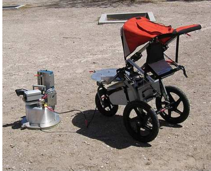
Figure 2. PI-SWERL (Portable In-Situ Wind Erosion Lab)
